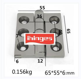
The IHINGES ML2-JL108 industrial hinge offers a compact yet heavyduty solution for equipment door mounting and enclosure applications. Crafted from durable 304 stainless steel with a mirrorpolished finish, this hinge is corrosion-resistant, aesthetically refined, and built to support up to 50kg per hinge.
