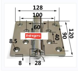
This heavy-duty industrial hinge is crafted from solid 304 stainless steel and engineered for high-strength applications such as large metal doors, equipment access panels, and heavy-duty enclosures.
