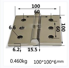
Model ML2-JL602-4R/L is a **removable pin industrial hinge** made from premium-grade 304 stainless steel. Measuring  $100\times100\times6$ mm and weighing 0.46kg, this hinge supports up to 60kg per piece and is designed for use on heavy-duty equipment doors, panels, and enclosures.
