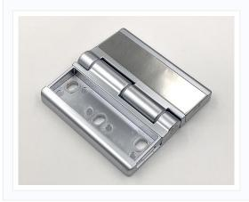
This is a heavy-duty hinge for use on industrial equipment such as industrial ovens, test chambers, and environmental test chambers. It has 6 mounting holes with oblong mounting holes for easy installation with minor adjustments. It is also equipped with a dustproof cover plate, which can be put on after installation to provide a good aesthetic effect. And there are nylon spacers added between the hinge blocks to the role of cushioning and improving the service life.
